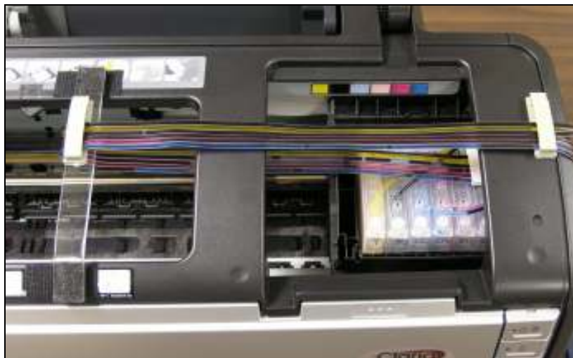
Proper tube installation
