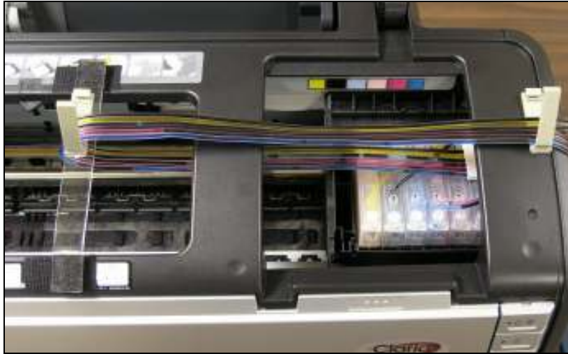
Guide the tubing through the clips so that it does not twist or flip
