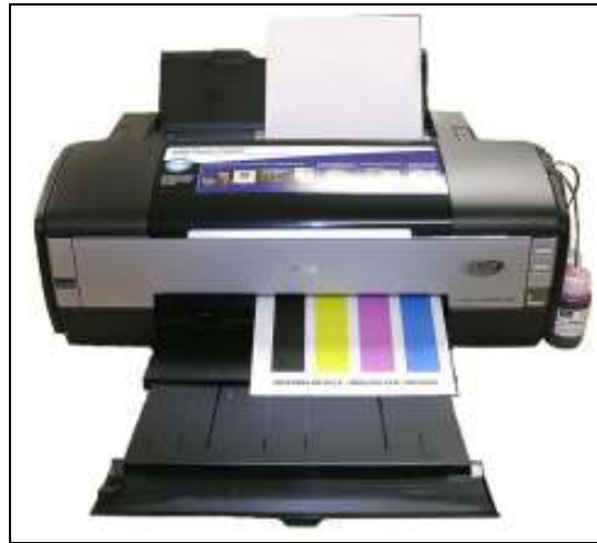
Epson 1400 with MIS CFS Installed
