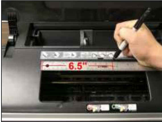
Place mark 6 1/2" from the left edge of the larger opening
